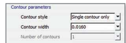
Figure 7: Contour width can be selected using a drop-down menu found in the Contour parameters options.
