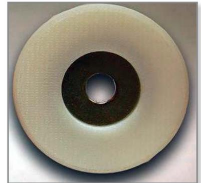
Figure 2: Embedded metal washer inserted into a 3D printed ABS part.
