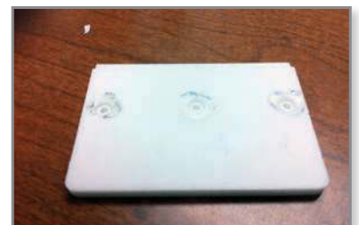
Figure 16: Spot welds from an ultrasonic welder.
