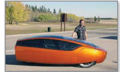
Figure 1: Full-sized car body used hot air welding and solvent to bond over 16 ABS-M30 ™ sections.
