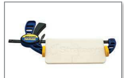
Figure 10: Align and clamp the mating pieces until the bond has set.
