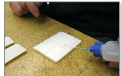
Figure 9: The low-viscosity solvent also flows well into seams and cracks.
