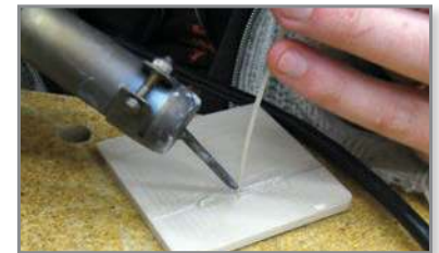
Figure 4: Draw the hot air welding tool and plastic filament along the seam.
