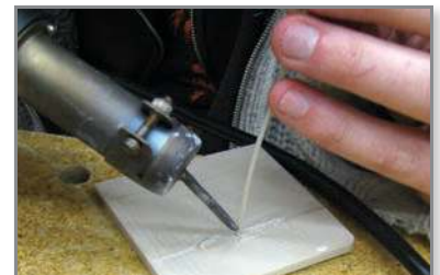
Figure 11: Hot air plastic welding.
