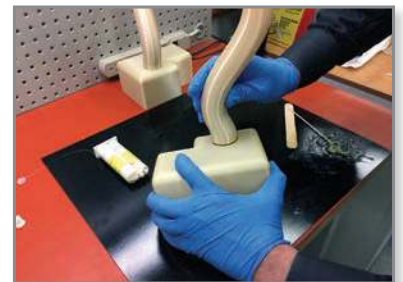
Figure 7: Mate pieces and hold or clamp.
