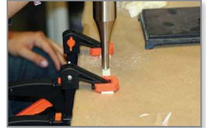
Figure 13: Clamp pieces for ultrasonic welding (ultrasonic horn shown).
