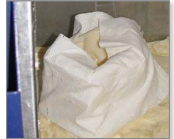
Wrap the part to absorb moisture and place it in the oven for 1 to 2 hours.
