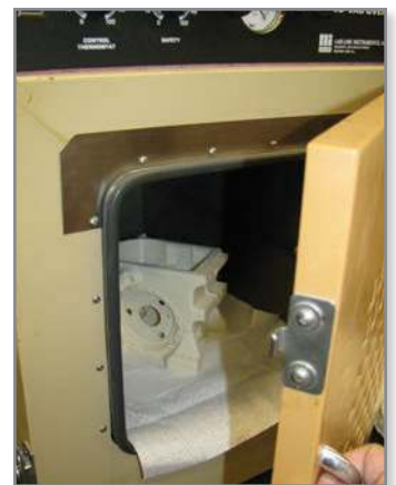
Use the vacuum chamber for multiple cycles to pull water out of the part.
