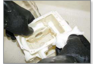
Rinsing the part is critical to remove any surface residue.
