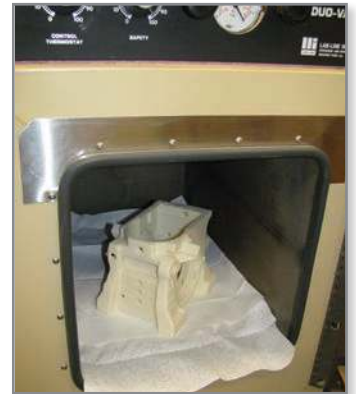
Use a liner or shop towel to absorb any excess water in the vacuum chamber.
