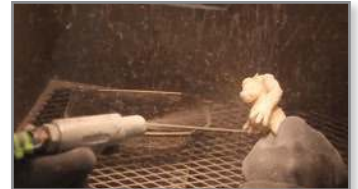
Figure 4: Media blast using a continuous, sweeping motion.
