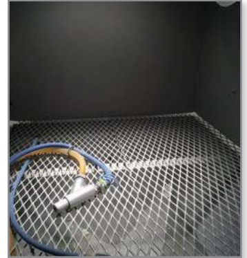
Figure 3: Place the part inside the blast chamber.
