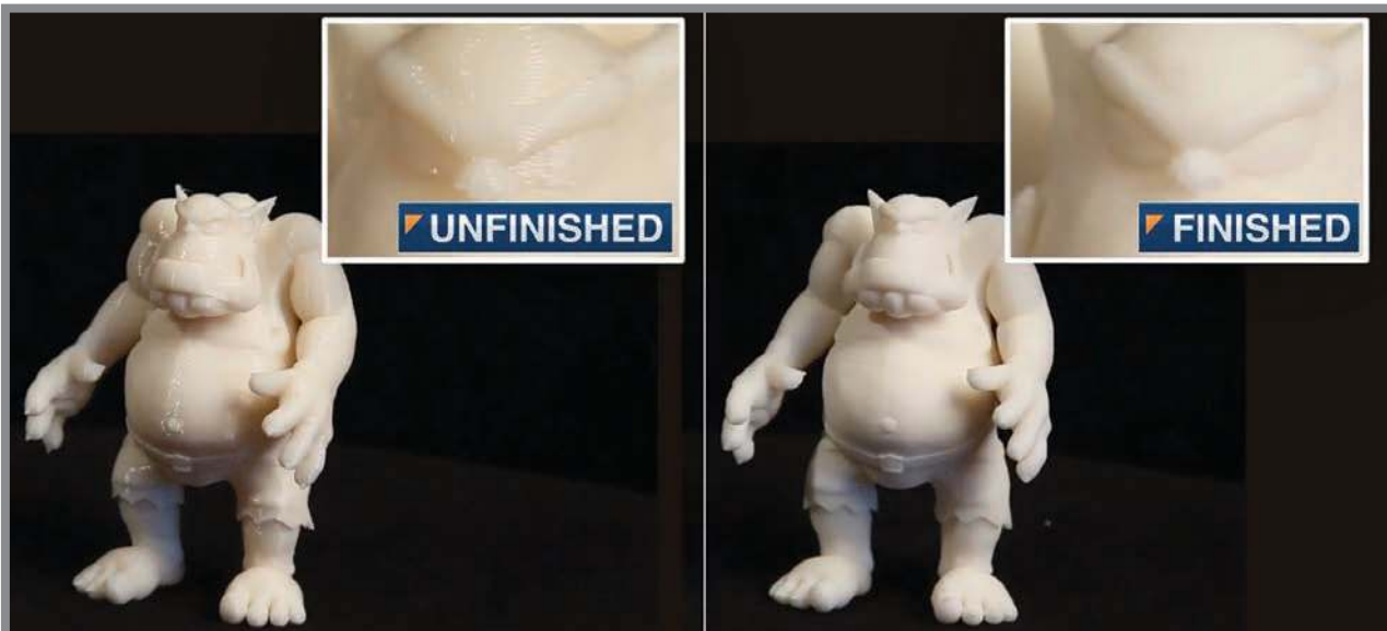
Figure 5: Unfinished FDM part (left); finished media-blasted part with smooth surfaces (right).
