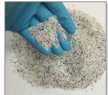
Figure 2: Plastic blast media is recommended for smoothing the surface of FDM parts.
