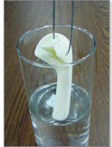
Figure 3: Dipping the part into solvent.
