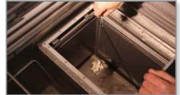
Figure 4: Transfer part to the smoothing chamber for a 15 to 30 second exposure.
