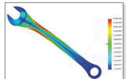
Figure 4: Output of a completed finite element analysis.
