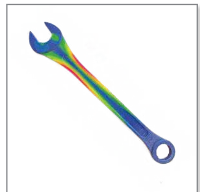
Figure 10: PolyJet model for hands-on review of FEA results.
