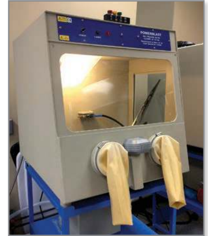
Figure 1: Removal of support material with a WaterJet station.
