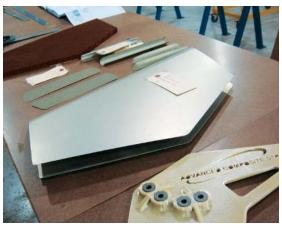
ACS helicopter fin (center) with AM drill guide (front).
