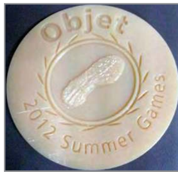
Figure 4: 3D printed model resulting from an STL file made using a BMP image.
