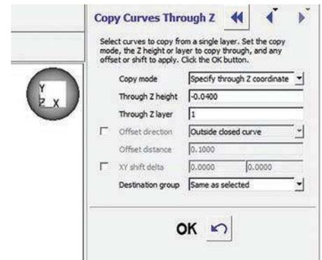
Figure 6: Extending the outer perimeter model contour to the build sheet using the Copy Curves Through Z options.
