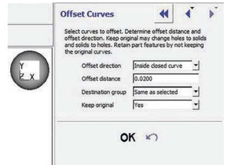
Figure 7: Offset the outer perimeter contour using the Offset Curves menu options.
