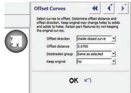
Figure 9: Offset all the support contours using the Offset Curves menu options.
