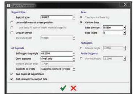
Figure 1: Support Parameters dialog box in Insight software.
