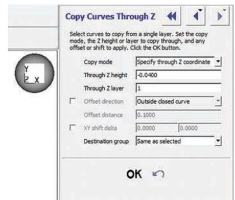
Figure 8: Extending the inner perimeter model contour using the Copy Curves Through Z menu options.
