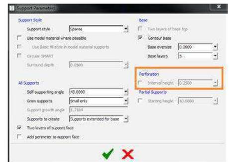
Figure 2: Clearing the checkbox in the Support Parameters dialog box to remove perforations.
