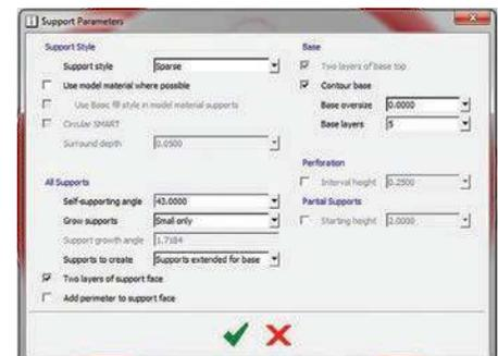
Figure 5: Ensuring the proper parameters are selected when generating supports in Insight software.
