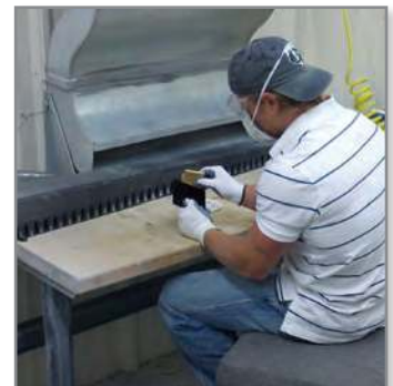
A worker sands ABS-ESD7 next to a dust-collection system while wearing safety glasses, gloves and a respirator.
