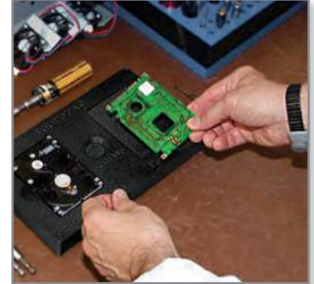
An assembly fixture for electronics made from ABS-ESD7.
