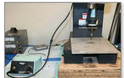
Figure 10: Press fitting arbor press.
