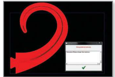
Figure 7: An Error Summary is displayed when a file that exceeds the build envelope is sliced
