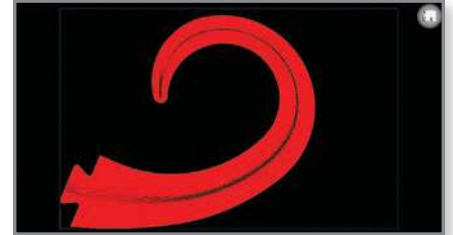
Figure 6: Part is oriented and sliced.
