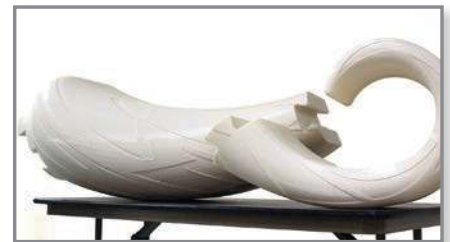
Figure 13: Oversized part that was sectioned in multiple places and printed on a Fortus 900mc™.
