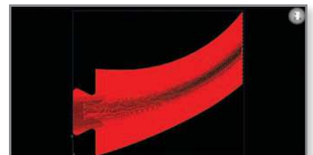
Figure 9: A registration feature is applied to the surface of the sectioned part.
