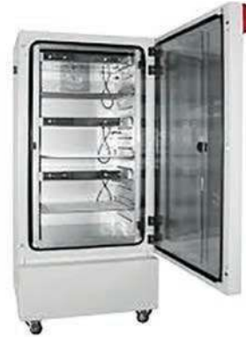
Figure 5: Illumination chamber for photobleaching.
