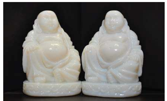
Figure 7: Rigur part before photobleaching (left) and after (right).
