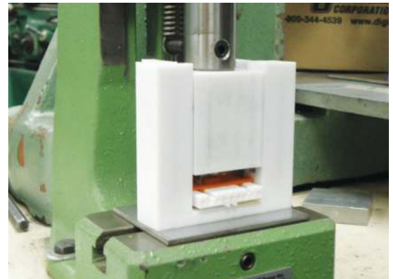
An operator at Xerox modified 350 connectors in about an hour on this toggle press.
