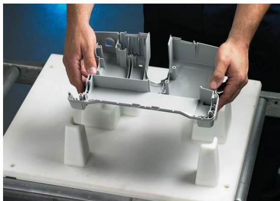
Oreck uses this jig during assembly of its vacuum cleaners. Here a vacuum top cover is placed into the pallet upside down.
