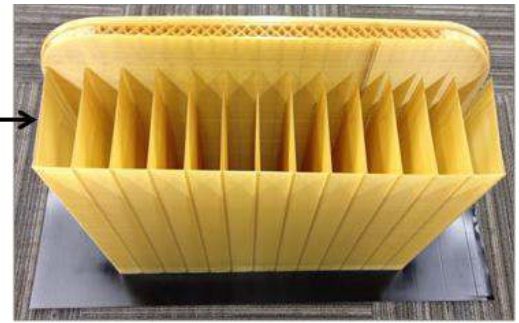
Figure 8-7: Composite tool printed with stabilizing walls indicated by the black arrow.
