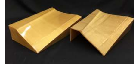
Figure 6-14: Sparse- and shell-style layup tools for UAV fan blades.
