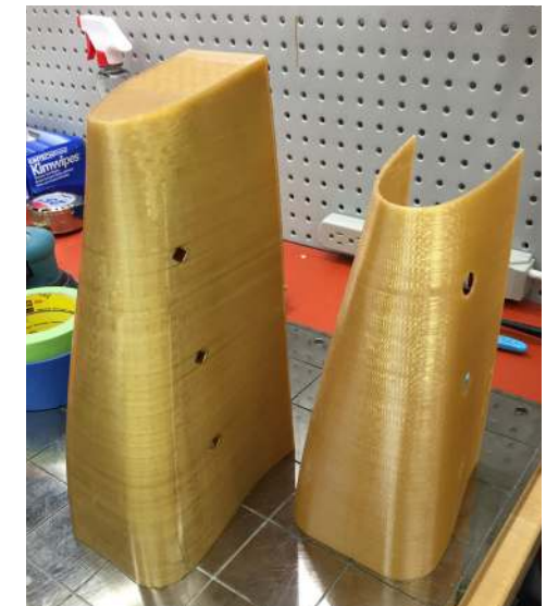
Figure 6-11: Shell-style shroud tool vertical build orientation (top); sparse-style lay-up tool and corresponding drill and trim tool (bottom).
