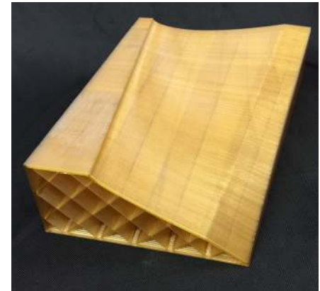
Figure 6-15: Sparse tool with large raster spacing and uncapped (open) ends.
