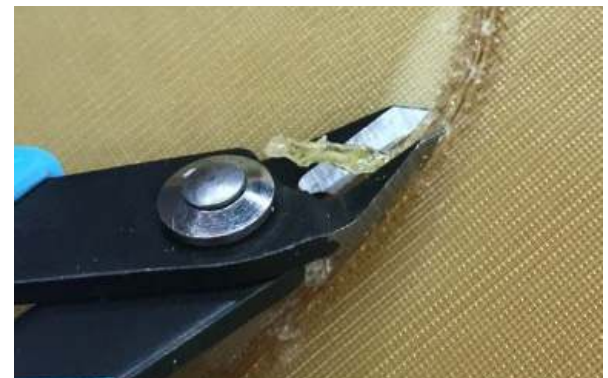
Figure A-6: Example of a poor bond because the filament can be easily removed.
