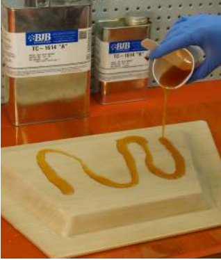
Figure B-4: Pouring epoxy on the tool.
