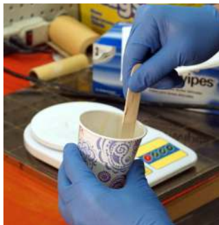
Figure B-3: Mixing the epoxy.
