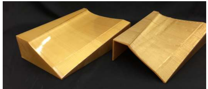
Figure 3-1: Sparse- and shell-style tools for a UAV fan blade.
