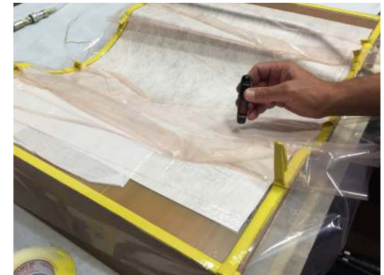
Figure 6-22: Vertical build orientation (top); vacuum-bagged part and tool during laminate fabrication (bottom).
