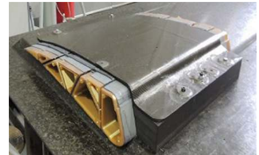
Figure 6-2: Aileron in-process lay-up and final configuration (vacuum bagging not shown).
