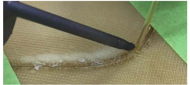
Figure A-5: Filament welding two sections together.
