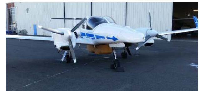
Figure 6-5: Composite belly pod fairing installed on Centaur aircraft (before and after painting).
