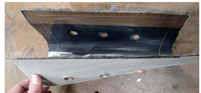
Figure 6-10: FDM tool in ULTEM 1010 resin (top) and resulting part (middle, bottom).
