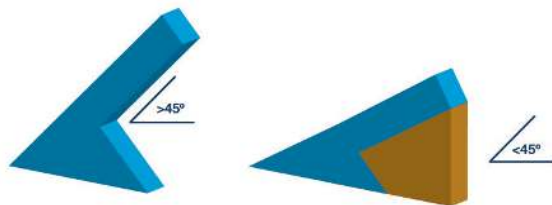
Figure C-5: Self-supporting angles (left) require no support material.
