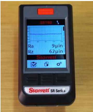
Figure B-8: Checking surface roughness with a profilometer.
