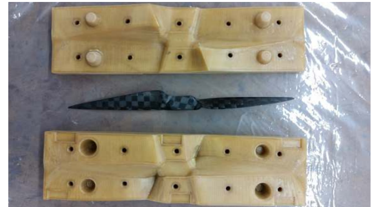
Figure 6-7: Carbon/epoxy composite propeller blade produced on a compression mold tool made from ULTEM 1010 resin
