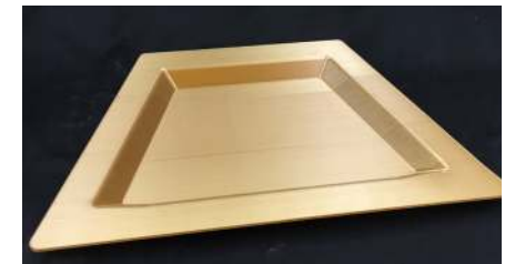
Figure 6-13: Pan skin vertical build orientation (top); top view of sealed tool (middle); the unfilled bottom surface of the tool with no post-processing (bottom).
