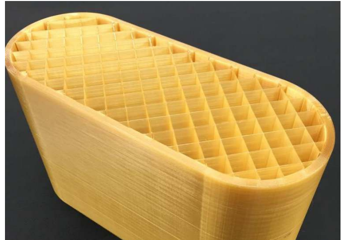
Figure 3-2: Test coupon for structural integrity testing of envelope-bagged, sparse style (sparse double dense in Insight), ULTEM 1010 resin. Raster spacing of 0.5 inch is shown.
