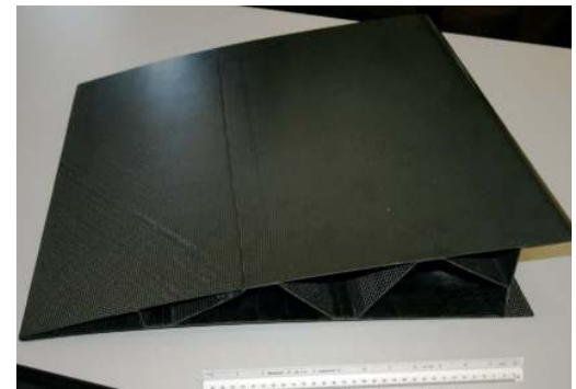
Figure 6-3: Final single shot composite aileron sub-scale demonstrator.
