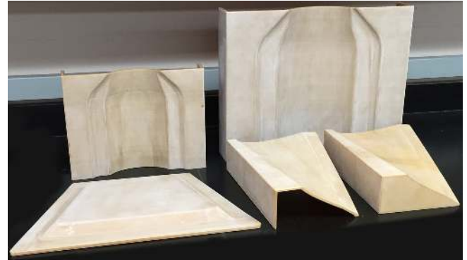
Figure 5-1: Tool designs used for thermal stability testing (shown sanded, but unsealed).
