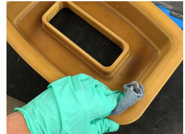
Figure 6-18: UAV bulkhead tool being prepped for use.
