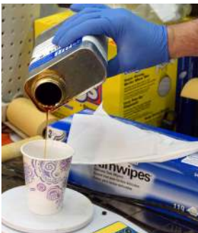
Figure B-2: Weighing the epoxy.
