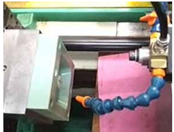
Figure 14: Cooling fixture mounted on the mold. As the mold opens, pressurized air is applied to the surface for a predetermined time.
