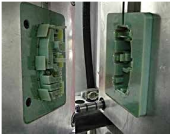
Figure 13: Mold inserts are assembled on a standard steel base and held in place with machine screws.
