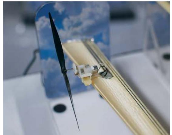
Aurora smart wing: 3D-printed structure with printed electronics.
