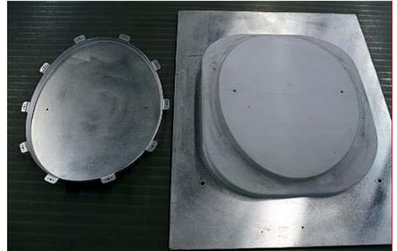
Piper Aircraft hydroforms sheet metal parts on FDM-created tools.
