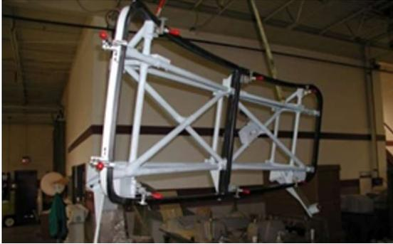
A cut-and-weld fixture for carrying a formed part.
