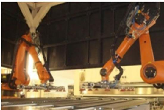
A twin robot assembly used to transfer flat metal blanks.
