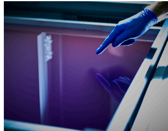
Stereolithography 3D printing technology uses a vat of liquid UV-curable photopolymer resin and a UV laser to build parts one layer at a time.
